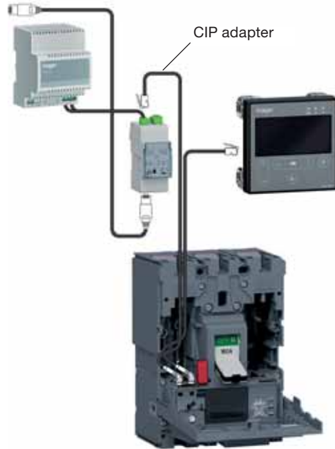
Modbus communication connection
