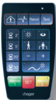
Infrared remote control EE807 to adjust the settings
